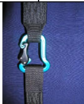
**The test setup is done with the DHV harness test bench, the application of the force to the brandnew carabiners/connecting elements was done with standardised harness belts.**
