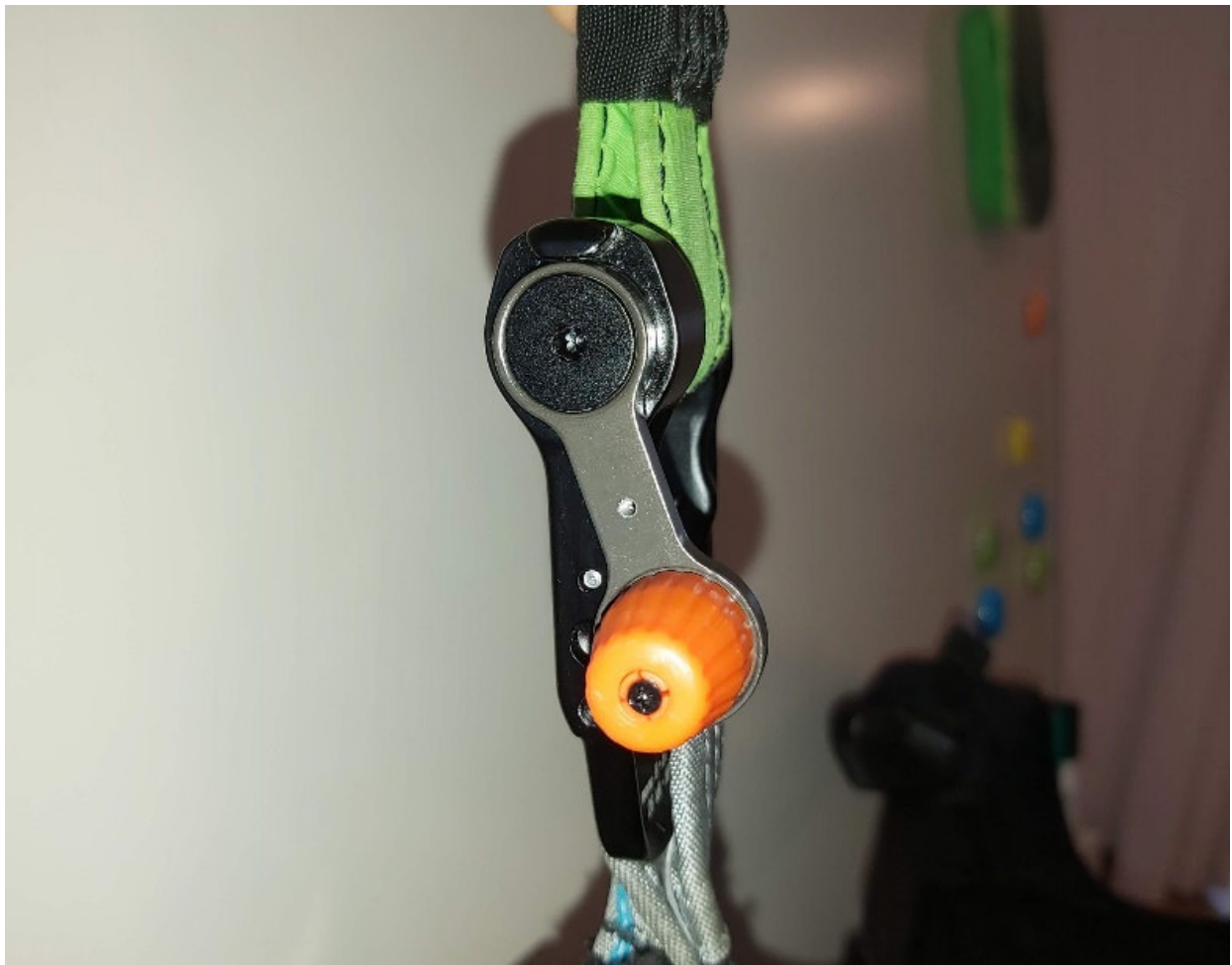
Release lever not snapped shut and locked into place.
