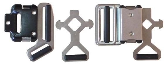
In the past three months, there have been two incidents involving older paraglider harnesses equipped with CLICK-LOCK buckles (HSi10) in the chest strap. The buckles had opened unintentionally during flight while they were under load. In one of the cases this happened during a SAT maneuver (spreading of the chest strap due to the pilot resting on the riser), in the other case the reason was presumably the load applied by the body weight of the pilot who was hanging only in the len straps.
