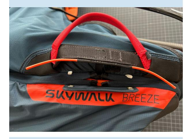
2. Tensile test on both rescue loops with 10 kg each.
