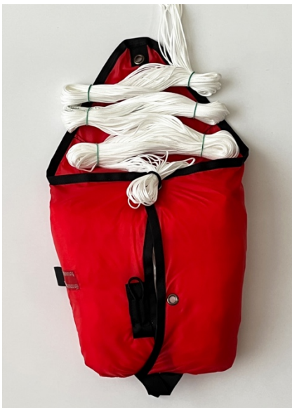
Opening of the top cover and release of the lines.
