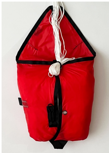
The canopy compartment remains closed until the lines are stretched.
