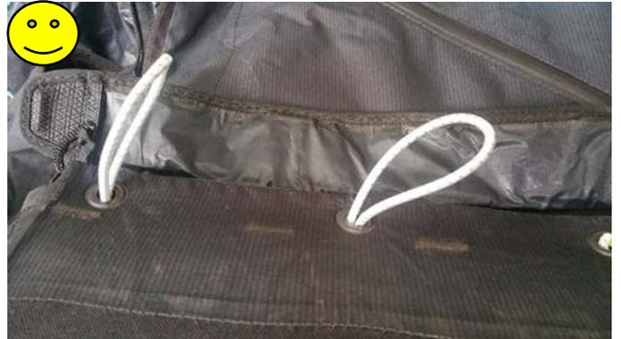
Both elastic loops may overextend, even if the rear one (the farther one from rescue handle location) is the most important one. Make sure the length of each elastic is does not exceed 8 cm.
