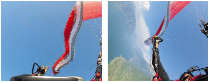
Mistral 7 gets a challenging collapse behaviour with massive collapses: severe dives forward, fast course change and collapses on the other wing side.
