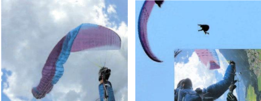
Even with collapses over the top limit of the LTF-field, Epsilon 7 behaviour was relatively moderate, with little dives forward and moderate curl of wingtip.
