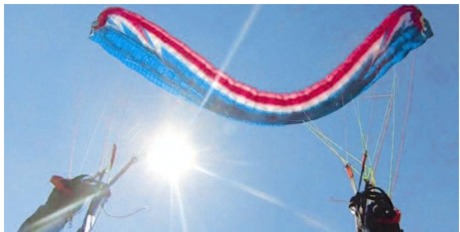
Spares the stable sink phase and deforms immediately on entry: Nova Mentor 3.
