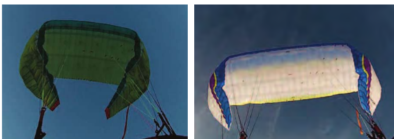
Large wingtip folds possible on the Mentor 4 (left). Pilot action required to recover. The wingtips on Airdesign's Rise 2 (right) tended to flap a little.
