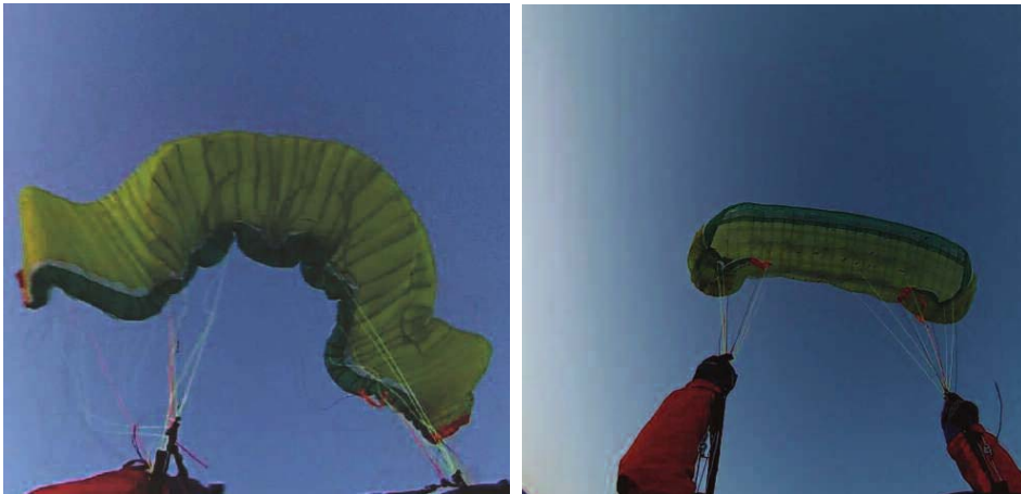
Nova Mentor 4: Again, massive collapses were difficult to induce, the canopy generally collapses at about 60% area. At the lower end of the weight range the canopy enters a short deep stall on recovery, but the folded wingtips help reduce forward dive dynamics.
