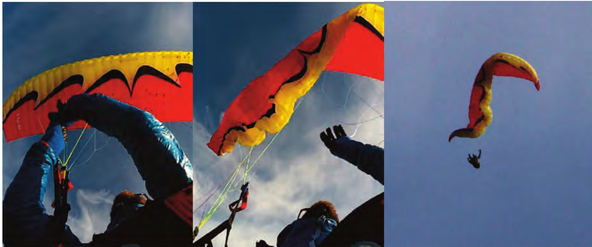
U-Turn Emotion 3: Both hands were required to produce high area steeply folded collapses. Recovery reactions were benign.
