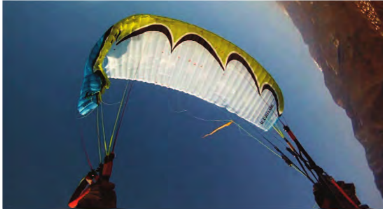
U-Turn Infinity 4: The picture shows how the leading edge may get caught in the lines after a collapse, at a point just behind the nylon rods. This sort of cravat is easy to recover from by applying gentle brake and does not result in continued rotation.
