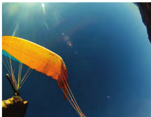
Advance Iota: the picture shows the slight cravat after an opposing collapse. The leading edge gets caught in the lines at a point at the end of the nylon rods. The cravat is simple to recover from with a little brake input, but sufficient to cause a rapid turn if left unattended.
