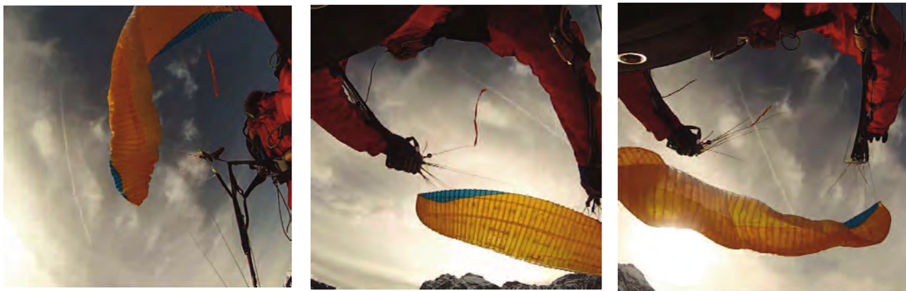
High area collapses at steep collapse angles (left) often opened impulsively during forward diving (middle). This increases the acceleration during forward pitching and results in a complete collapse of the leading edge (right). Recovery from this was fast, did not cravat and required no pilot input.
