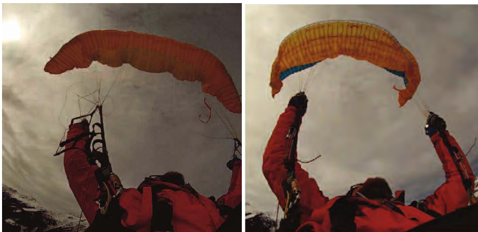
Advance Iota: behaviour is normal for the gliders classification. At the lower end of the weight range recovery is slightly delayed. Re-inflation is progressive from the canopy mid-point outwards, and recovery rapid with marked forward pitching.
