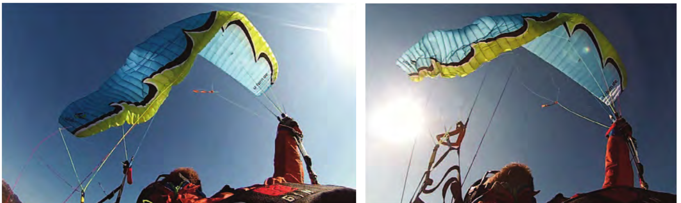
U-Turn Infinity 4: Steep folding angles are accompanied by high area collapses and dynamic recovery reactions. Reactions to smaller collapses are more benign.
