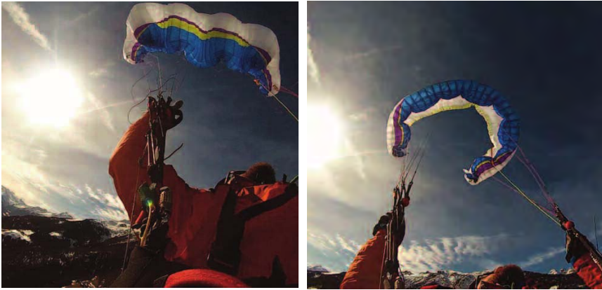
Airdesign Rise 2: Massive collapses were difficult to induce. Generally the glider collapses at about 60% area. On massive collapses at the lower end of the weight range (left) recovery was slightly delayed (right), but the glider self re-inflated progressively from the middle.
