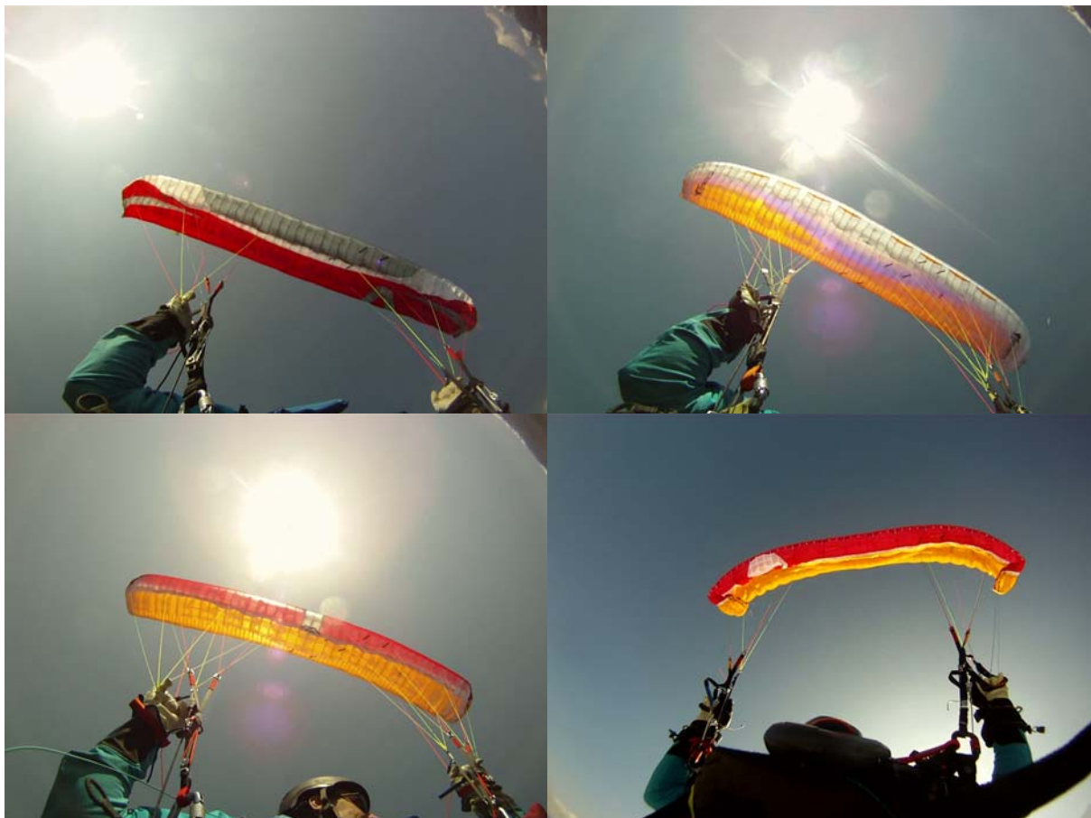
B-Stalls are not a problem for Skywalks Chili 3 (top left), Icaros Wildcat TE (top right) and Mac Paras Eden 5 (bottom left). Wingtips deform after a few seconds on Gradients Nevada (bottom right).
