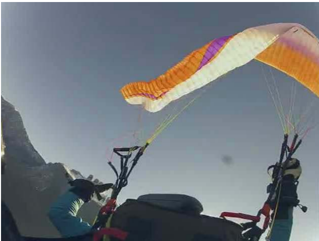
Assymetric collapse on an Icaro Wildcat TE. Compared with the Eden 5 and Nevada, this glider reacts more dynamically to deformations. Total height loss was not more than for other gliders.
