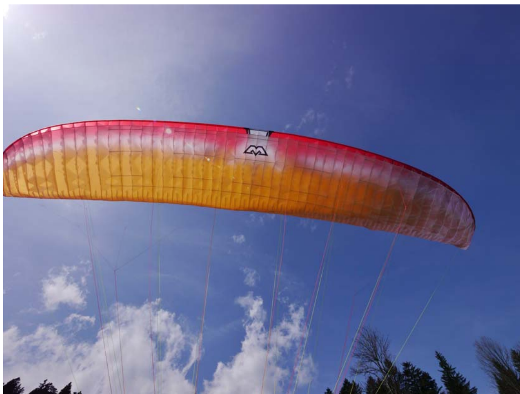
Picture: The high-end B segment is packed full of high-tech: mini-ribs, diverse horizontal tapes, plastic rods at the nose and C-lines and aspect ratios approaching 6. Pictured is the Mac Para Eden 5.
