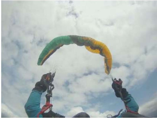
Ozone Mojo 4 (right) recovers delayed after a front collapse, Sky Paragliders Anakis 2 (left) recovers very quickly.
