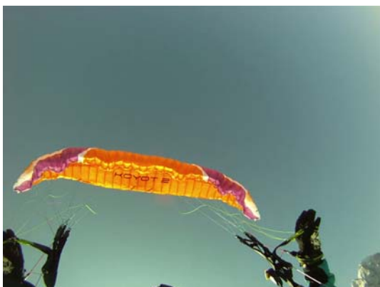
Small collapses are unspectacular on Niviuks Koyot 2 whereas larger ones display a tendency to severely delayed recovery.
