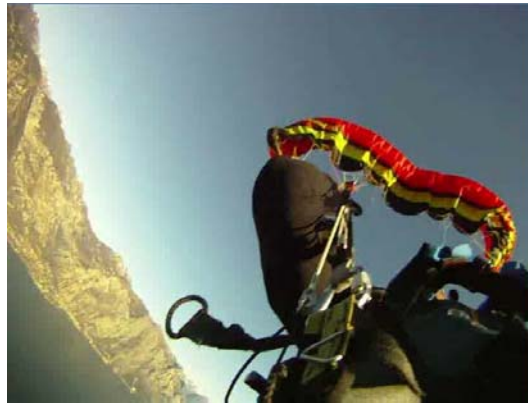
These gliders tend to fold in the middle on a hard front collapse and may recover asymmetrically: Independence Pioneer (right). Reduced tendency on the Icaro Cyber TE (left).
