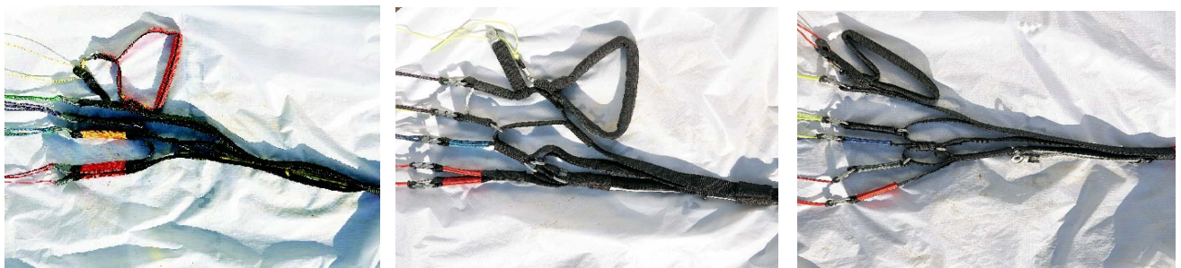
Pictures: The Sky Anakis 2 riser (left) is light and uncomplicated but very soft. This makes handling more difficult. Unusual: The Brummel hooks for the speed system is attached to the inside of the A-riser. On the Vita from Air Design (middle) risers are made of thick but soft webbing with a total of 4 metal speed system rings, and need a little getting used to. Swings Arcus 7 has standard risers with nothing unusual about them (left).
