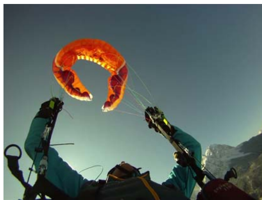
Small collapses are unspectacular on Niviuks Koyot 2 whereas larger ones display a tendency to severely delayed recovery.
