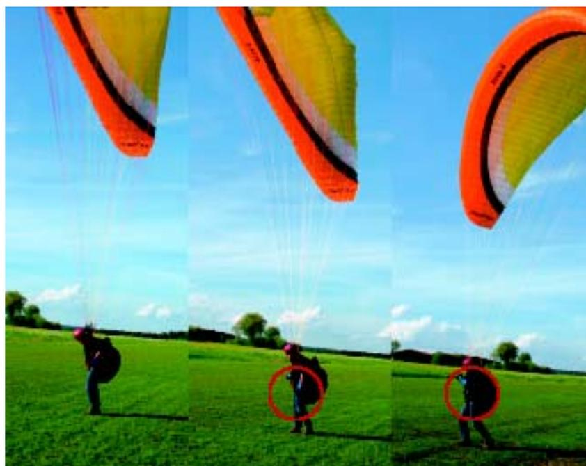
Ask a colleague to collapse the canopy on one side by pulling on the outside A-lines. You will realise by how much the pressure on the affected control line decreases. Try to be quicker than your colleague and prevent/reduce the collapse by correcting the control pressure immediately. In order for that to work, the collapse must be induced by a small impulse only and not by keeping the A-risers pulled down. Otherwise it won't work.
