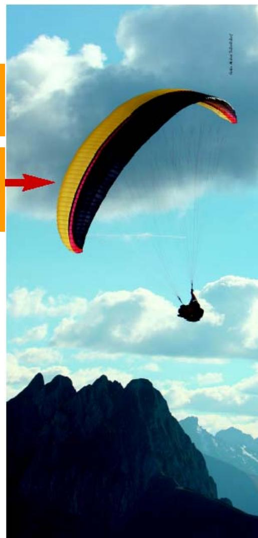
Paragliders are strange flying objects, so strange indeed, that the usual laws of aerodynamics that normally apply in aviation, fail to explain everything that can happen to this wing. This flying object whose centre of gravity is located seven to eight metres lower than the wing and is also continuously moving back and forth, cannot be explained by the classic rules of aerodynamics alone.
