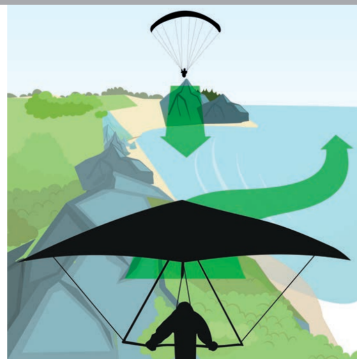
Soaring above the ridge: The glider with the Lee to the left should give way to the right.
