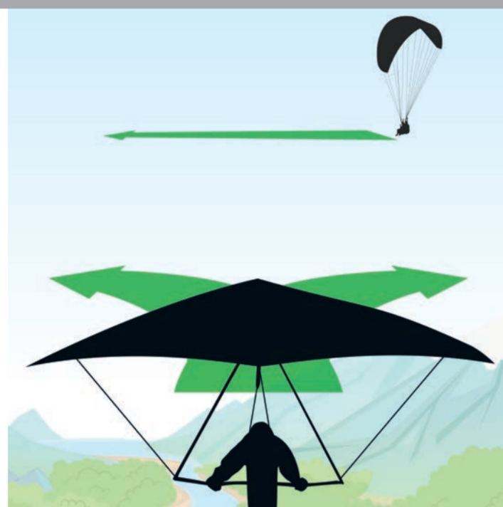
Converging course: The aircraft that has the other on its right must give way.
