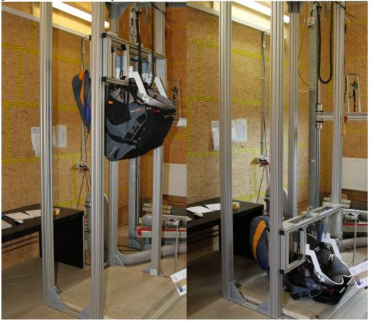
Current protector testing according to the LTF. Protector damping is measured after impact from 165cm (dummy base to floor). The deceleration (G) acting vertically on the spine is measured at impact. Limits: Maximum 50G must not be exceeded, a period of 7 ms must not bee exceeded at 38G and a period of 25ms must not be exceeded at 20G. Current testing simulates a pilot crashing vertically on his / her bottom.
